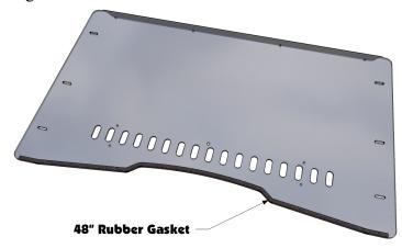
3. Next install the sliding vent panels on the inside of the windshield as shown in the diagram below. To install slide fasteners push through holes with thumbs until it is completely through the hole in the windshield and locked in place.
