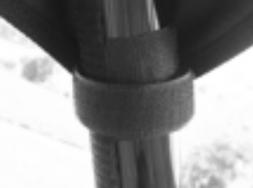
4. While locating the positions for the adhesive Velcro the best place to start is the front corner. Place a 6" adhesive Velcro strip at the bottom of the front roll cage as shown in the picture on the next page.
