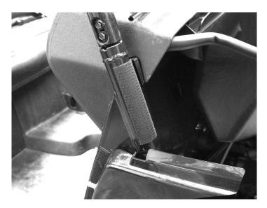
5. Now install the 16" long 1" wide adhesive Velcro strip down the front of the fender as shown below.
