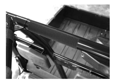
10. Now take the rear window and attach the two 8" tabs to the adhesive Velcro centering the cutout across the top under the rear brake light. The photo below shows how it should look.
