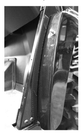
6. After the Velcro is placed at the bottom of the roll cage and along the fender line attach the front of the door to place it where it needs to be. This helps to assure that all the remaining Velcro will be at the correct locations to hang the door right. The photo on the next page shows how the front of the door should look.
