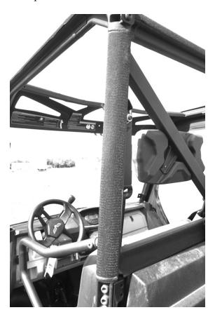
5. Now attach the Rear window to the frame making sure to center it correctly. When installing the doors the rear part of the door will attach to the sides of the Rear Window.
