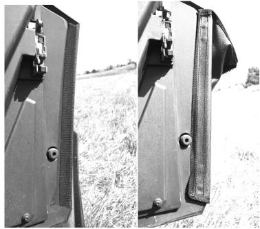
12. Lastly install the snap studs into the plastic for the bottom rear portion of thee door. It works best to put the screw studs into the snap sockets on the door first. Then one by one pull the door in place and push the screw into the plastic making sure to put enough pressure to leave a mark. Then remove the screw stud from the door and install it where the mark was left behind at. The following picture show what it looks like.
