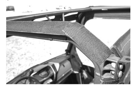
9. After all the Velcro is in place take the door and place it on the vehicle. The following series of photos show how it should look after being installed.
