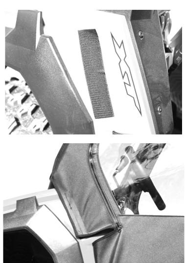
11. Now take the 18" Strip that is 1" wide and place it on the inside front portion of the factory door. Then take the bottom front section of the soft door and wrap it around the factory door and attach the two together as shown in the photos below.
