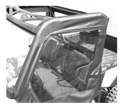
10. Next attach the 8" adhesive Velcro strip to the bottom of the front top portion of the door as shown in the photos below.
