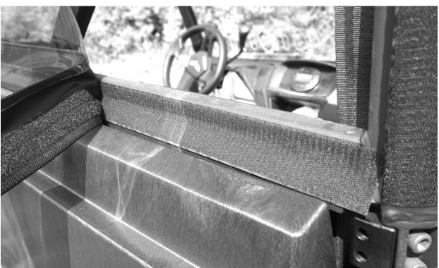
4. Next install the 20" adhesive strips down each side of the Rear Window as shown in the photo below.
