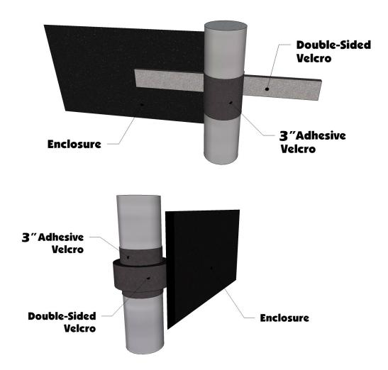
2. Next take the 8" and a 12" adhesive Velcro strips and run it down the back of the roll cage facing towards the rear of the vehicle. They should match up with the double-sided Velcro tabs sewn along the rear of the soft door. See photo below.
