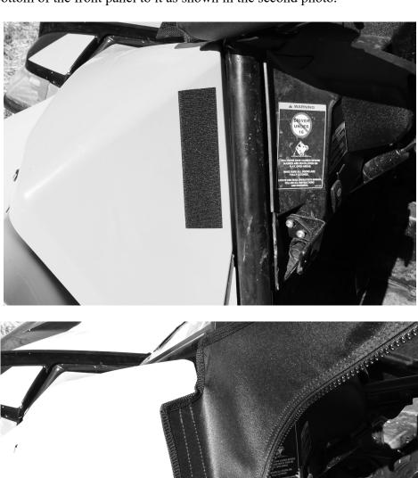
4. Last part of the door to attach is the bottom to the factory half-door. Take the 44" adhesive Velcro strip and attach it to the factory door to match up with the Velcro sewn to the bottom of the soft doors. The adhesive Velcro will cross the hinge of the door, take a knife and cut the adhesive Velcro at the hinge. See the following photos.
