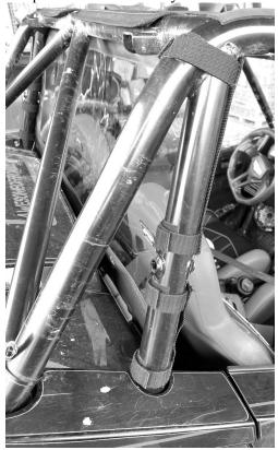
3. Finally attach the two 6" and the one 18" adhesive strips across the bottom of the Rear window behind the seats. See pictures below
