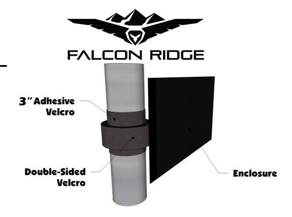
2. Once all the double-sided Velcro strips are attached all that is left is to attach the adhesive Velcro that matches up with the Velcro sewn along the bottom of the door. The rear part of the door will use the 13" adhesive strips that will go on the vehicle as shown in the picture below.
