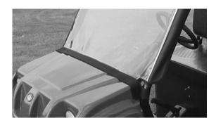
4. Working your way to the rear of the roll cage carefully fit the Cab into position. Lift the rear bed and pull the rear of the cab down and make sure the top of the cab is tight to the roll cage. Now mark the locations for the four 6" adhesive Velcro strips across the bottom of the cab and attach.
