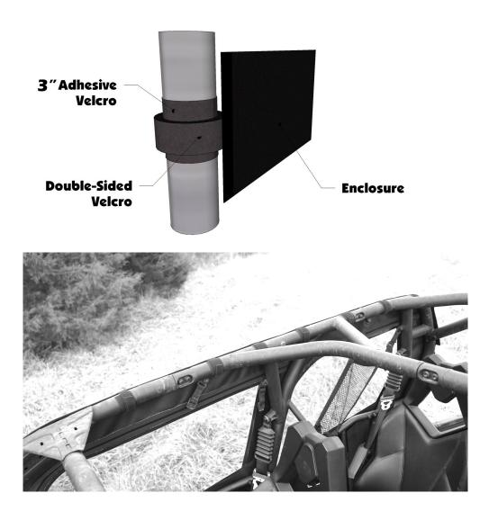
4. Next take the 30" adhesive Velcro strip and run it down the back of the roll cage facing towards the rear of the vehicle. They should match up with the double-sided Velcro tabs sewn along the rear of the soft door. See photo below.
