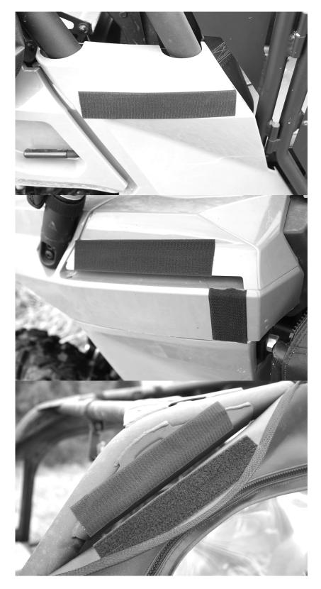
6. Last part of the door to attach is the bottom to the factory Pro Armor half-doors. Take the 8", 20" and 25" adhesive Velcro strips and attach it to the factory door to match up with the Velcro sewn to the bottom of the soft doors. The adhesive Velcro will be on both sides of the hinge on the door.
