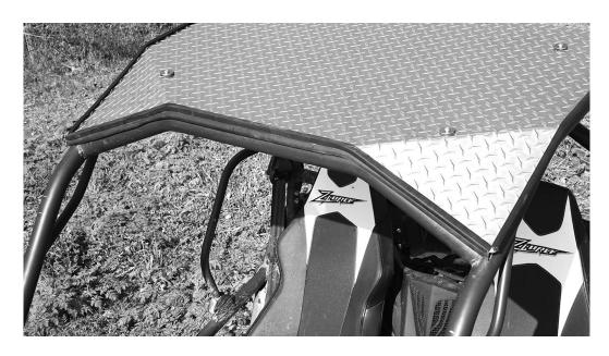
3. Next place the roof on the vehicle and attach it to the frame. You will see six tabs on the frame. Bolt it on with the 1" bolt and large stainless and rubber washers on the outside and large stainless washer and lock nut on the underside. See photos on next page.
