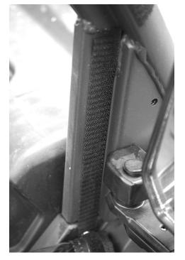
9. Lastly install the snap studs into the plastic for the bottom portion of the door. It works best to put the screw studs into the snap sockets on the door first. Then one by one pull the door in place and push the screw into the plastic making sure to put enough pressure to leave a mark. Then remove the screw stud from the door and install it where the mark was left behind at. The following pictures show what it looks like.
