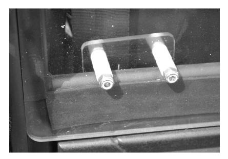
10. Once the Rear Window is in place and properly centered on the vehicle the final step is to install the brackets across the top of the window to secure it in place. This is done the same as the bottom brackets except you use the white nylon washers and 1 1/4" bolts. See photos below.
