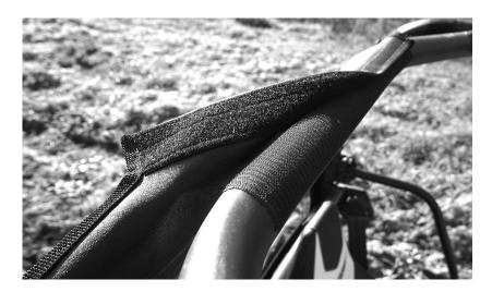
2. Next take the 20" adhesive Velcro strips and run it down the back of the roll cage facing towards the rear of the vehicle. Start at the bottom and work your way up the bar. See photo on next page.
