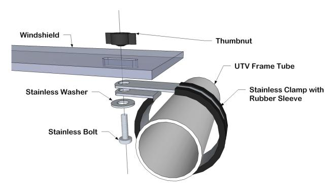
6. The four clamps that hold the windshield across the top use the large stainless and rubber washers to hold the windshield on. The inside part of it uses a small washer and a lock nut. the following photo shows how it should look.
