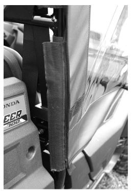
6. Now move to the front lower corner and place the 9" adhesive strip to match up with the Velcro on the cab. See photo on next page.
