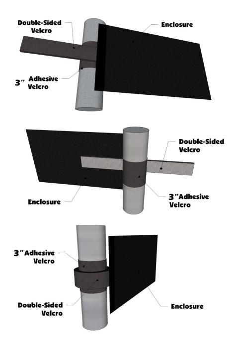
5. After attaching the double-sided strips go to the rear of the door. You will see three Velcro tabs sewn here. Starting just below the top cross bar place the 32" adhesive strips down the bar facing the rear of the vehicle. Then pull the tabs around and attach then down the bar to the Velcro. See photos on next page.
