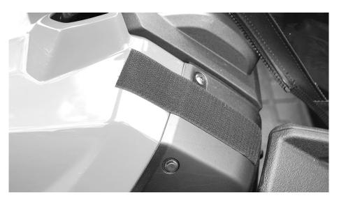
7. Last item on the doors will be a snap on the inside front section of the plastic doors. It's easier to place the snap in the right position by first putting the screw snap stud into the socket on the enclosure. Then pull the door into place and push the snap into the plastic so that a mark is left. Then pull the snap out and screw it into the door making sure not to over tighten and strip out the plastic. See Photos Below.
