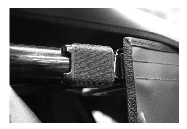
12. Then take the Rear Door and zip it to the Middle Rear Window. This ensures the door is properly placed. Then attach the top front corner to the Velcro. See photo below.
