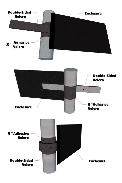
5. After attaching the double-sided strips go to the rear of the door. You will see three Velcro tabs sewn here. Starting just below the top cross bar place the 32" adhesive strips down the bar facing the rear of the vehicle. Then pull the tabs around and attach then down the bar to the Velcro. See Photos below.
