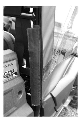
6. Now move to the front lower corner and place the 9" adhesive strip to match up with the Velcro on the cab. See photo on next page.
