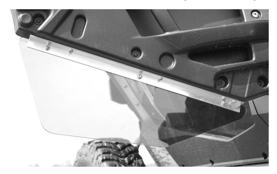
6. The rear door panels use the short angles and attach to the panels using the side with three holes with the holes of the other side of the angle towards the larger end of the panels as shown in the photo below.
