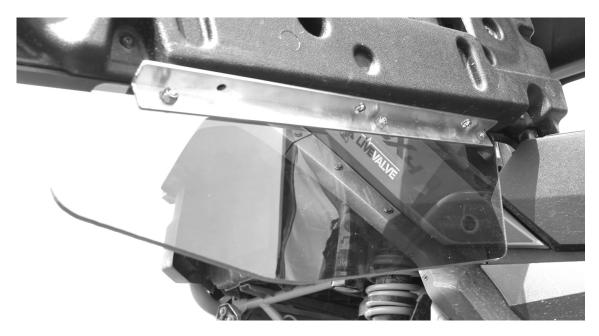
7. Now shut the doors and place the panel under the door so that it fits in the space and mark the bottom of the door where to drill holes to attach it.
