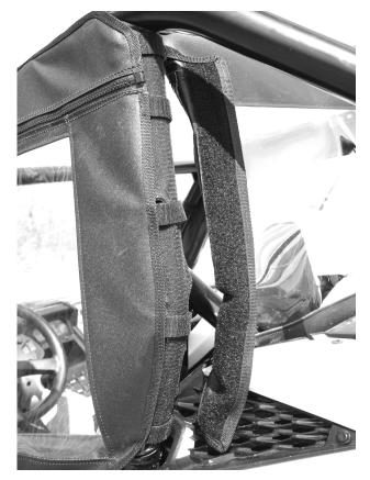
4. Lastly place the two 12" adhesive hook strips behind the seats as shown in the picture below.
