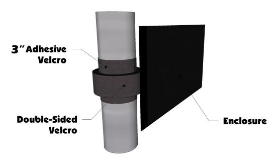
**5.** When you get to the back of the door, take the 20" adhesive strips and place them down the roll cage so it faces the rear of the vehicle. Then wrap the double-sided strips around the bar as shown in the picture below.
