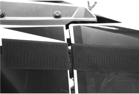
**9.** Next place the 6" adhesive strips on the vehicle to match up with the front portion of the door as shown in the photo below.
