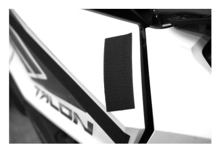
10. Lastly place the other 6" adhesive strips on the vehicle to match up with the Velcro on the very front bottom part of the door as shown below.
