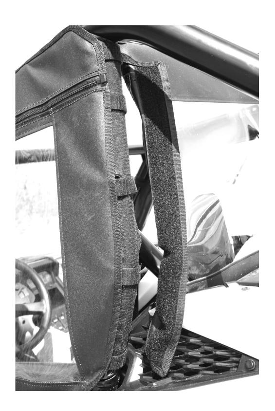
**6.** After attaching the double-sided strips go to the bottom of the door. Pull the bottom of the door up and place the 40" adhesive strip on the Velcro sewn to the door. Leave the paper backing on it as you put it on then peel it off after getting it in place. See Photos below.
