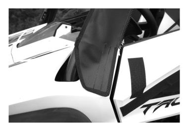
11. Along the top of the Rear Window you will see 6 double-sided Velcro strips. At each of these, place a 3" adhesive hook strip in the inside of the roll cage. This holds the double-sided strip in place. See images below
