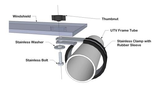
5. Along the bottom use the two 1 ½" clamps the attach the rear window as you did along the sides. The following pictures show where all the clamps go.
