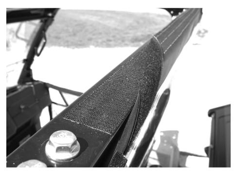
4. Next place the 45" strip on the rear vertical bar. It should be placed on the outside of the bars along the back edge. See photo below
