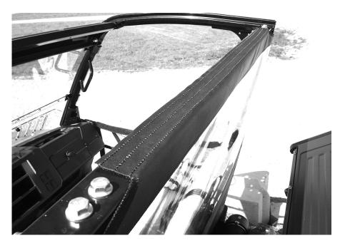
7. Now attach both sides of the Rear Window to the adhesive Velcro strips down the outside of the rear corner bars as shown in the photo below.
