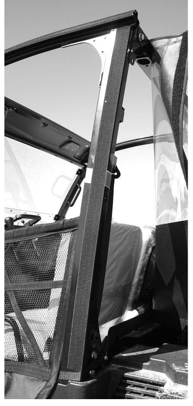
5. Last piece of adhesive Velcro goes at the bottom of the Rear Window along the plastic piece. Place the 36" strip centered on the plastic piece facing towards the rear of the vehicle. See photo below
