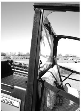
8. Then just push the bottom of the Rear Window against the Velcro strip across the bottom as shown in the photo below.
