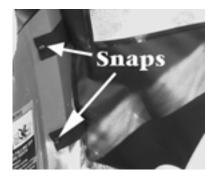
11. To open and stow the doors, move the zipper fully rearward and fold the bottom portion of the doors up. Then begin to form a vertical roll with the door by rolling it inward from the front edge toward the rear of the door. Secure in place using the two hook and loop straps provided. Try to form a roll approximately 2" in diameter to assure that the door will not stick out very far while stowed.
