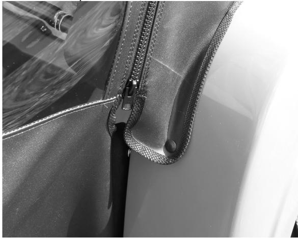
10. Finally install the two snaps on the inside of the fender as shown below.
