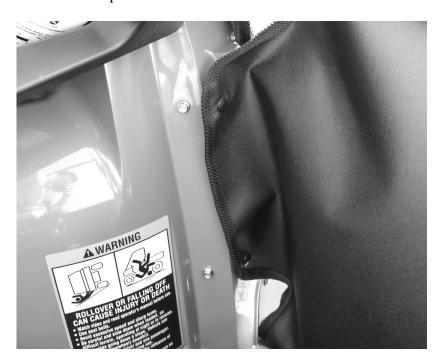
11. Rear Window: Begin by placing the 20" adhesive Velcro strip across the top bar. It should be placed toward the top and front of the vehicle. Then attach the top of the Rear Window to the Velcro as shown in the photo below.
