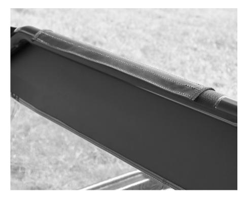
12. The bottom of the Rear Window has magnets that should now the attached to the metal strip.
