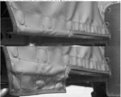
8. Now install the snaps for the front lower portion of the doors. Start with the strap sewn in the front corner as shown below.
