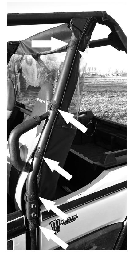
4. Last thing to do for the Rear Window is to attach the straps along the bottom to the frame of the seat under the bottom cushion. The following picture shows how it should look.
