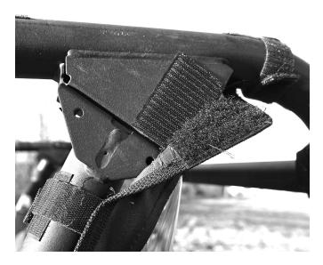
2. Next hang the Rear Window from these adhesive strips making sure to center the window properly. Once this is done attach the two double-sided Velcro strips at the very top corner of the Rear Window. Make sure to pull the top of the Rear Window tight from side to side. At each double-sided Velcro strip you will use one 3" adhesive strip to keep the double-sided strip from moving. The following pictures show how this is done as well as a picture of the Rear Window after it has been attached.
