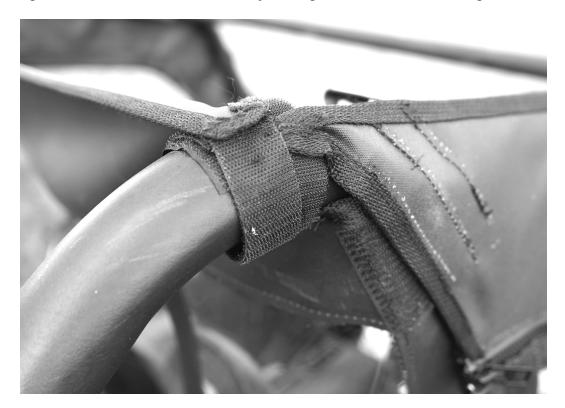
8. Finally, the bottom of the door has Velcro sewn across the entire length. Place the 30" adhesive Velcro strip on the outside of the door to match up with the bottom of the soft door. Also, the front corner has a 10" piece of Velcro running vertical. See photo below.
