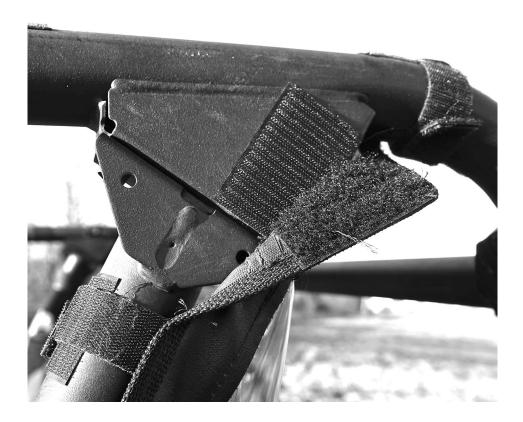
6. Now line the door up with the frame and begin attaching the double-sided Velcro strips as you did with the sides of the Rear Window. Photo below shows where they are.
