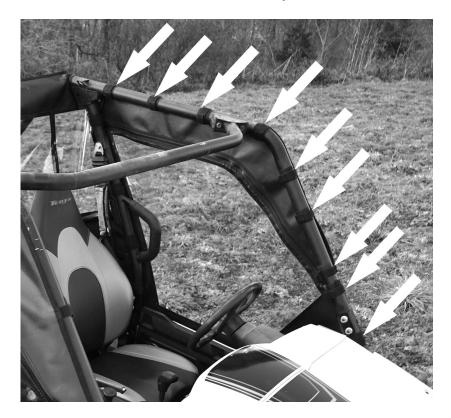
7. After you have the front and top double-sided strips attached you can now attach the strip at the very top rear corner of the door. If you have the Rear Window on it is very likely that the two will be at the same location or right next to each other. This is fine, just wrap one over the other. See photo below.
