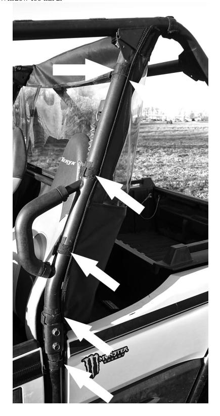
4. Last thing to do for the Rear Window is to attach the 14" Velcro strips and straps along the bottom to the frame of the seat under the bottom cushion. The following picture shows how it should look.
