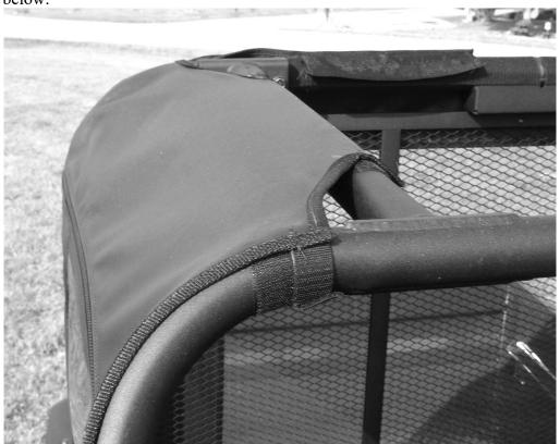
5. Now work your way down the front first placing 3" adhesive Velcro on the inside of the roll cage where each of the double-sided strips are sewn to the edge of the door. The diagrams below show how this works.
