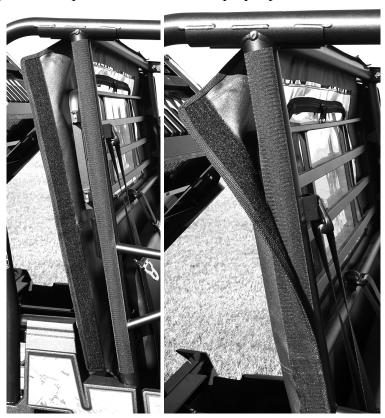
3. The bottom of the Rear Window is held in place by the 63" adhesive Velcro strip and the two 6" strips. The 63" strip goes across the bottom on the plastic from one side to the other. The two 6" strips hold the bottom of the sides on each side. The adhesive strips go on the very bottom end of the roll cage. The photos below show what it should look like.
