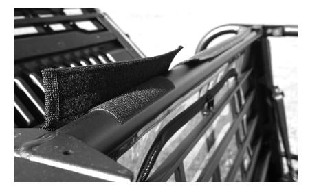
2. Next place the two 35" adhesive Velcro strips down the side bars. There is really only one space that this strip can fit, and it is just behind the side protection bars and to the outside of the brackets that hold the rear cage panel in place. The photo below shows the proper placement.
