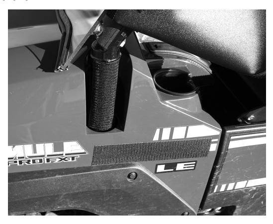
8. Finally, the bottom of the door has Velcro sewn across the entire length. Place the 25" adhesive Velcro strip on the outside of the door to match up with the bottom of the soft door. See photo below.
