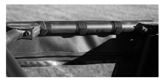
5. The rear edge of the doors has a strip of Velcro sewn down the entire length. This attaches to the Velcro sewn down the sides of the rear window. Magnets in the top rear corner hold it in place against the roll cage. See photos below.
