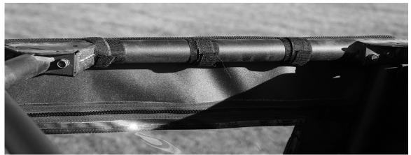
3. The rear edge of the front door also has double-sided strips as well, but you do not use the 3" adhesive strips for it. Instead place the 45" adhesive strips down the backside of the middle bar facing the rear of the vehicle. You will need to cut the adhesive strip and place part of it above and below the mount for the bar as shown in the photo. This will hold both the double-sided straps and the sides of the middle rear window in place. See photo below.
