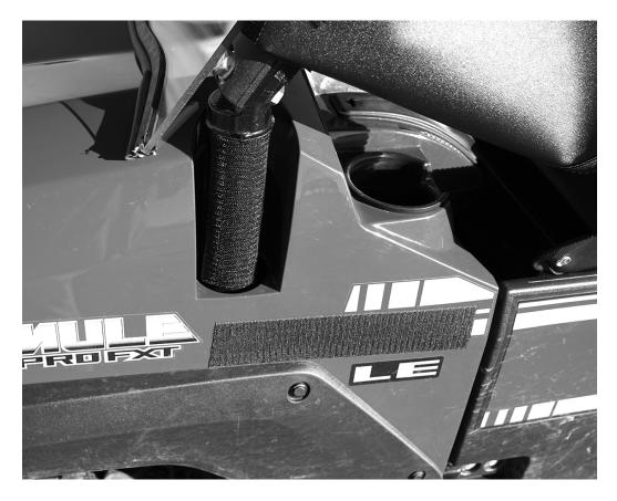
6. Finish off the bottom of the Door with the 25" adhesive Velcro Strip. See photo below.
