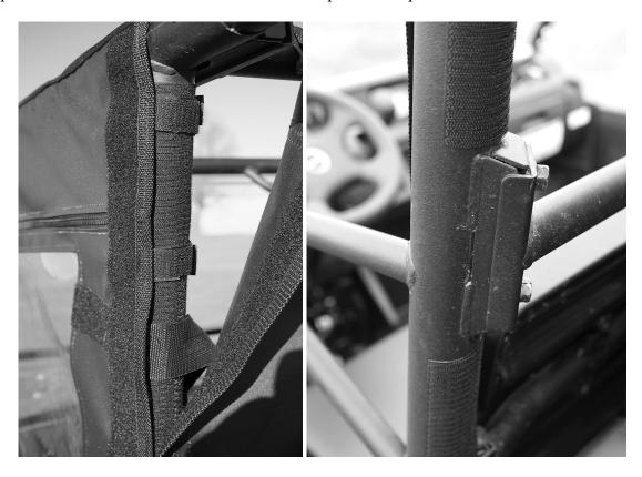
4. The diagrams below show how the double-sided straps and the 3" adhesive Velcro works.
