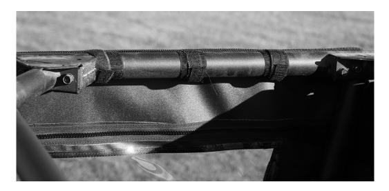
5. The rear edge of the front door also has double-sided strips as well but you do not use the 3" adhesive strips for it. Instead place the 45" adhesive strips down the backside of the middle bar facing the rear of the vehicle. You will need to cut the adhesive strip and place part of it above and below the mount for the bar as shown in the photo. This will hold both the double-sided straps and the sides of the middle rear window in place. See photo below.
