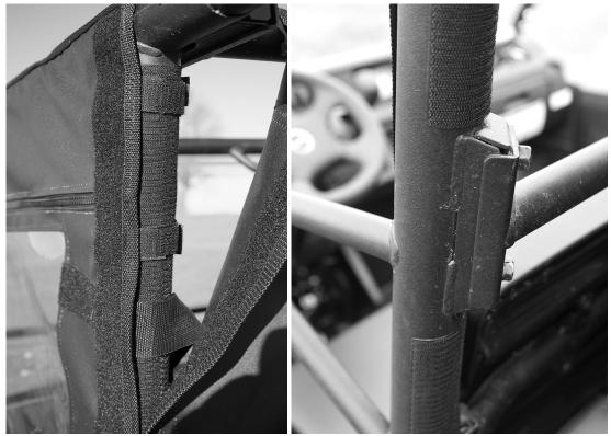
6. The diagrams below show how the double-sided straps and the 3" adhesive Velcro works.
