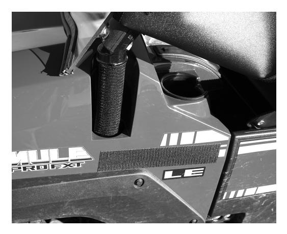
8. Finish off the bottom of the Door with the 25" adhesive Velcro Strip. See photo below.
