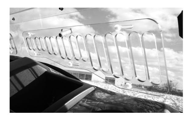
6. Now install the lower portion to the upper portion using the nylon bolts. There are five holes in both section with the holes in the upper portion being bigger. Set the upper portion on top of the lower portion and screw them together making sure that the slots on the ends are lined up. The photo below shows how this looks.
