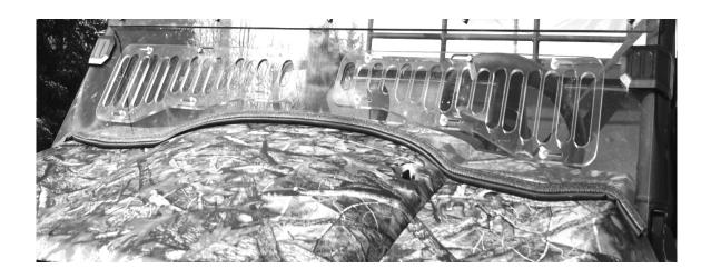
4. Next prepare the vent slider to be installed on the windshield. Take the 2" bolt, Black nylon spacers and lock nut and attach them to the vent sliders as shown in the photos below.
