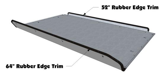
1. Run the edge trim from the channel on one side around to the channel on the other. See photo below.
