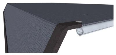
2. Next attach the front section of the roof to the vehicle using the 1 7/8" clamps, Rubber Washers, Large Washers, Small washers and a Lock Nut. These should be used along the sides of the roof with two on each side. The hardware should be attached as shown in the photo below.
