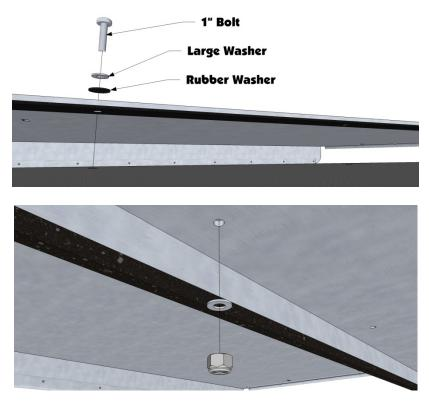
5. The holes on the ends are to be used to attach the bent bolt covers. Attach them as shown in the photo below.
