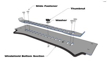
5. Next take the bent Lexan brace and install it on the outside of the windshield. The bend will be above the bolts when installed. Please refer to the diagram below.
