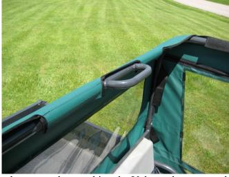
• Now hang the cab from these spots by attaching the Velcro tabs sewn to the cab enclosure in these spots. It may be necessary to remove and reattach the tabs until the cab is centered correctly.
