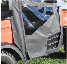
• To open and stow the doors, move the zipper fully rearward and fold the bottom portion of the doors up. Then begin to form a vertical roll with the door by rolling it inward from
