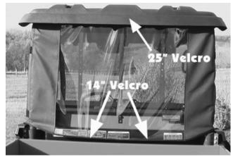
6. You will see six double-sided Velcro strips along the sides. At each location use one of the 3" adhesive Velcro strips on the inside of the roll cage then wrap the double-sided strips around the roll cage to lock it in place. See diagrams below.
