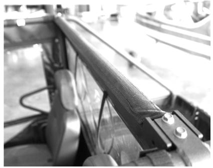
3. Then place the Rear Window on the window by centering the panel and attach at the top first then the sides. See photo below.
