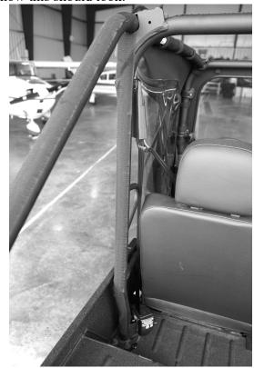
2. Now take the remaining 45" adhesive Velcro strip and run it across the top of the top rear bar as shown in the photo below.
