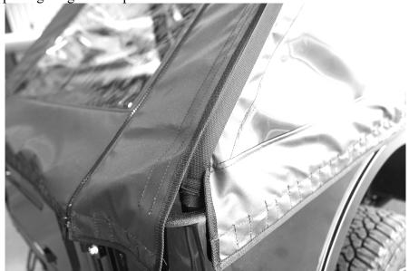
4. Once all the straps are in place run them through the buckles. Pull them tight making sure the top is centered and the side seams line up correctly along the roll cage. The diagram below shows how to lace the webbing through the buckle.
