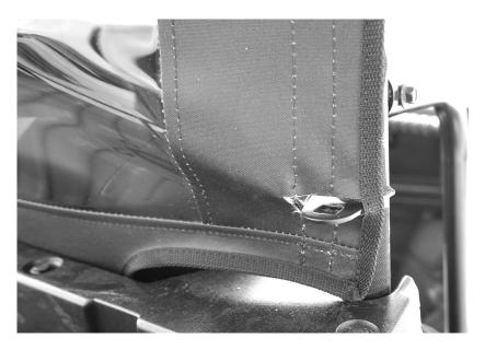
6. Lastly take the 30" adhesive Velcro strip and place it on the wall behind the seats to match up with the Velcro sewn along the bottom of the Rear Window
