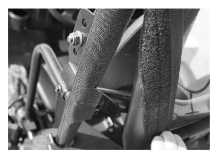
5. On the passenger side there is a slit in the Velcro, this is where the Flag mount will go through. See photo below:
