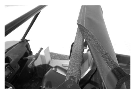
4. The sides attach to the bars using the 20" adhesive Velcro strips. On the passenger side you will need to cut the Velcro and place it above and below the flag mount. See photo below.
