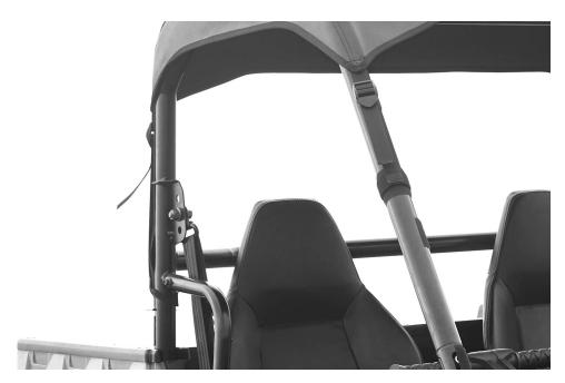
4. Now run the looped end of one of the strap around the roll cage just under the top of the safety bar on the side. Then pull the other end of the strap through the loop and pull tight. Photo below shows how it should look.
