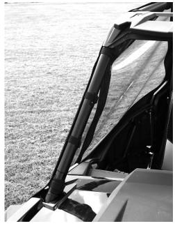
b. After installing the double-sided strips move to the top of the door and attach the 37" adhesive hook strip starting at the front and work it on the bar towards the rear. The strip will start on the side of the bar and end up on top of the bar at the rear. See Photo Below:
