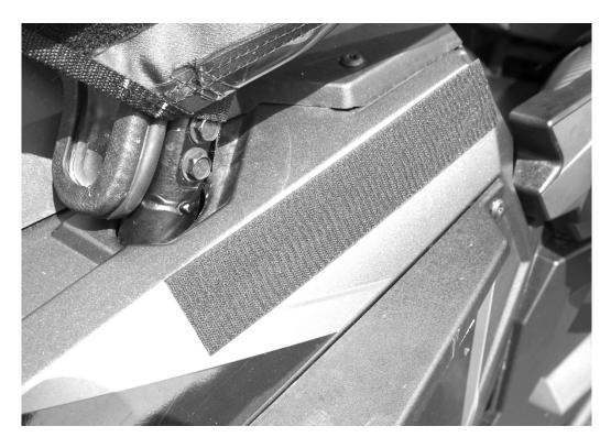
d. Lastly attach the two flaps on the inside of the door to the inside of the metal frame of the factory door. These pieces are there to hold the bottom of the door in place when the door is rolled down so it doesn't fall away from the door. See photo below
