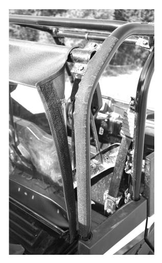
5. Next take the 15" adhesive Velcro strip and place it along the top of the small rear side panels as shown in the photo on the next page. Then affix the bottom of the rear panel to it as shown in the second photo.
