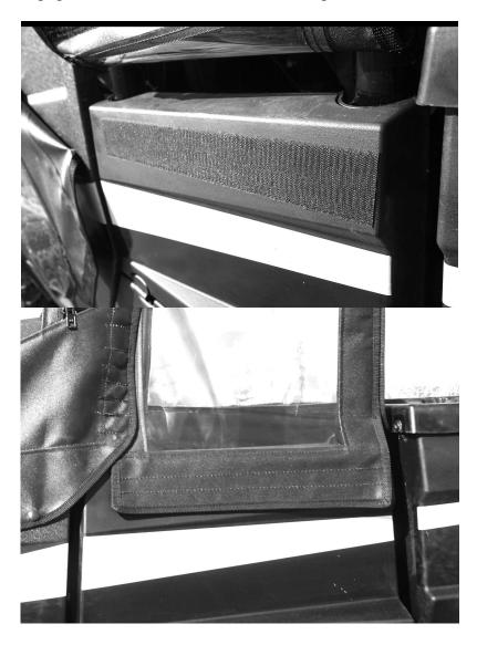
6. Next place a 3" adhesive strip on the center bar towards the bottom of the rear panel to match up with the double-sided strip as shown in the photo below.
