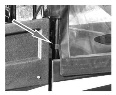
7. Last piece of Velcro is the 3" strip on the end of the front strip as shown in the photo on the next page.
