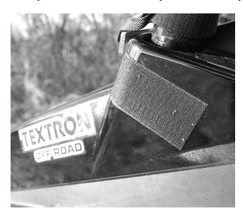
8. Once all the Velcro is in place the last thing to do is install the screw snap studs. NOTE: The best way to install the snap studs is to put them in the sockets in the door first. Then push them into the plastic to make a mark. Then pull the screw stud out and screw it into the plastic where the mark was made. See Photo Below.
