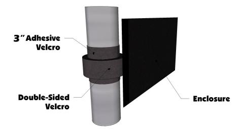
4. Next take the 30" adhesive Velcro strips and run it down the back of the roll cage facing towards the rear of the vehicle. Start at the bottom and work your way up the bar. You will see the double-sided Velcro tabs sewn along the back of the doors that will attach to this strip. See photo below.
