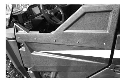
9. Final step on the doors are to install the polycarbonate panel in the hole at the bottom of the factory half door. Take the panel screws and install the panel on the inside of the door as shown in the pictures below.
