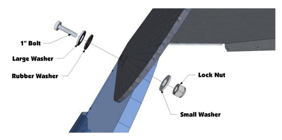
7. Make sure that the top and windshield are straight with each other. The bolt should fit in the middle of the slot on the roof. When together they should look like the photo below.
